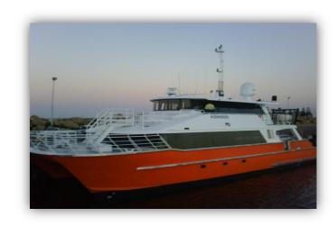
Komodo is a 24.8m catamaran utility vessel especially designed and modified to conduct extended environmental, oceanographic and geophysical survey and operations at sea. She has accommodation for 18 personnel, and can be equipped with dive spread, chamber, A-frame, winch and tender.
