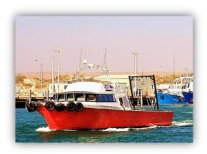
VG is a modern design utility vessel of single chine planning hull configuration. Construction is in heavy duty welded marine grade aluminum with welded aluminum superstructure, incorporating a fly bridge driving station. The vessel is classed under the USL code in WA and the Northern Territory for coastal operations to 200 nautical miles offshore.
