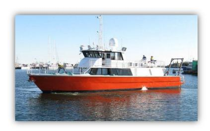
Calypso is a 24 m specialised vessel purposely designed for extended offshore marine survey and environmental research. Calypso has accommodation for twelve personnel, and is equipped with A-frame, AIS, winch and tender. Calypso can also be equipped with dive spread and chamber, as was required for recent conduct of the Gorgon Marine Environmental Baseline Programme (the vessel was dedicated to between October 2007 and 2012).
