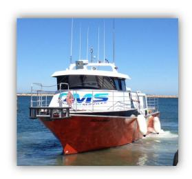
Ocean Spirit is a modern design high speed jet powered utility vessel. She is a single chine planning mono-hull. She has a raised bridge to facilitate excellent visibility from the helm position. The vessel is classed under the USL code in WA for coastal operations to 100 nautical miles offshore.
